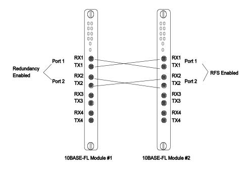
Figure 3-4. 10BASE-FL Modules Connected with Redundancy/RFS Enabled
